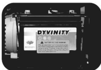
STEP 2. Connect the battery before starting.
