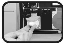
STEP 10. Connecting the load.
