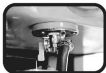
STEP 6. Turn the fuel switch on.
